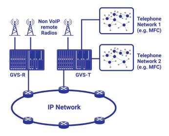
Thanks to their modularity, GVS devices can be customized to cope with small radio sites up to large radio installations with tens of co-located radios through a number of possible interfaces (4 wires standard E&M analogue, E1, Nx64, QSIG digital, etc.). The same applies on the telephone side, where multiple co-existing connections to different telephone networks are provided as a standard option.
