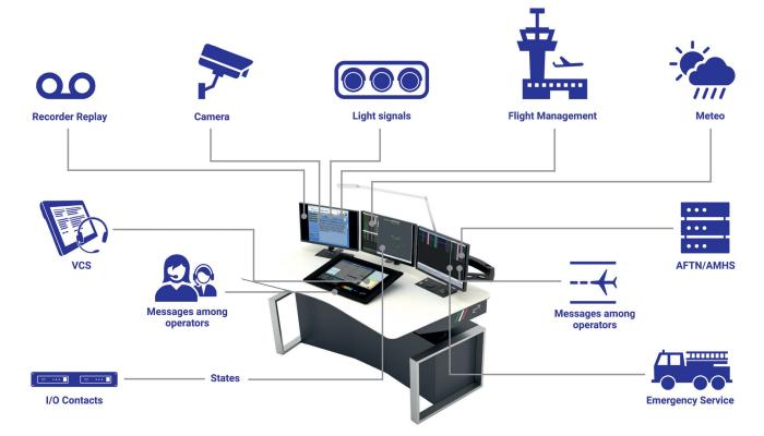
MTF800 Integrated Information System is a hardware/ software platform for Airports of any size or Remote Towers which concentrates different data sources into one integrated product with the aim of reducing the number of objects on the operative desks, and whereas increasing the operator's situational awareness while attending to their duties.
