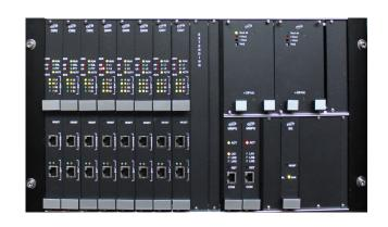
GVS devices include facilities to automatically look for other radios with the same characteristics in case of failure of the one being used. This automatic search procedure allows VCS operators to continue their work without suffering of service disruption, even in case of total radio failure. Best Signal Selection (BSS), audio compression and delay compensation are standard features provided by GVS devices.
