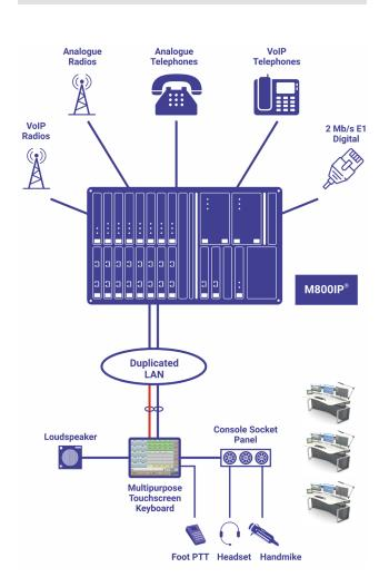
All telephone and radio interfaces are contained in a single drawer with duplicated power supply, providing access to:
