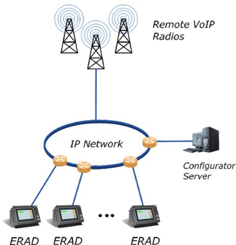
ERAD mounts a 7-inch touch-screen and has head-phone/microphone/PTT inputs that enable it to function as a complete operating position. Thanks to the internal gateway, it connects autonomously to a WAN or LAN based on the IP protocol.
